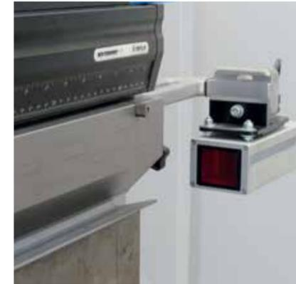
Allows the operator to work safely close to the tools even as the RAM and backgauge moves at high speed. The maximum speed holds up to 6 mm distance from the part. The system continuously monitors the speed performance of the pressing beam.
